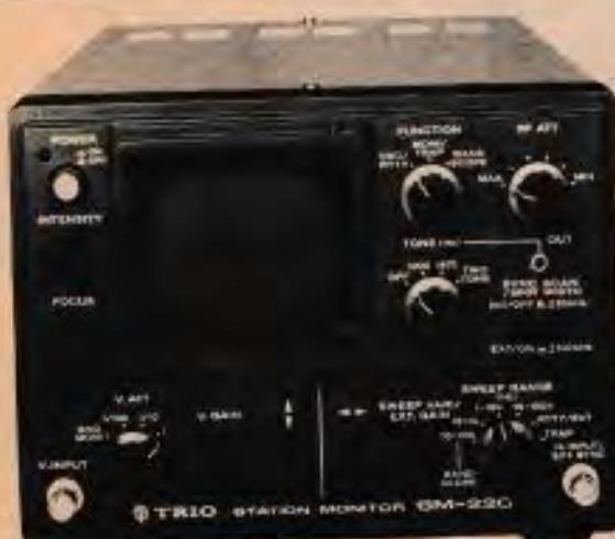
Based on a wide-frequency-range oscillator (up to 10 MHz), the SM-220 station monitor features, in combination with a built-in two-tone generator, a wide variety of waveform-measuring capabilities. An optional feature is a unique pan-display capability. The SM-220 provides efficient visual operation in monitoring transmitted waveforms, and it also serves as a high-sensitivity, wide-frequency-range oscilloscope for various adjustments and experiments.
