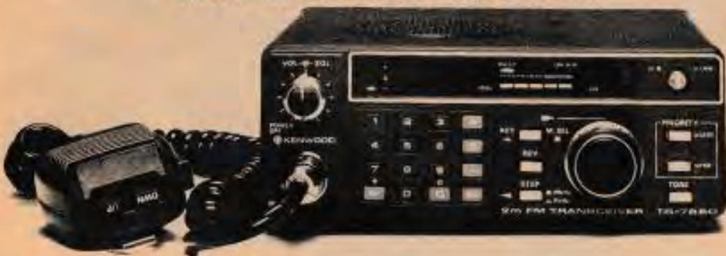
Kenwood's remarkable TR-7800 2-meter FM mobile transceiver provides all the features you could desire for maximum operating enjoyment. Frequency selection is easier than ever, and the rig incorporates new memory developments for repeater shift, priority, and scan, and includes a built-in autopatch DTMF encoder.
