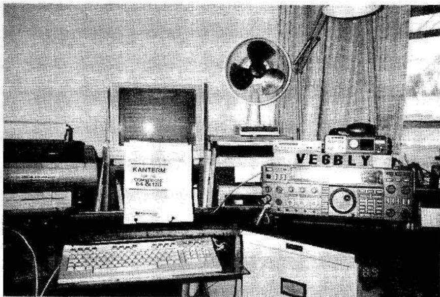
All Mode Amateur Radio Station: Left to right, top, Star SC10C printer on 1571 disk drive, 1902A RGB monitor, 1541 disk drive under fan and paper rack. Kantronics KAM left top of Icom 761 and Yaesu 227R 2M beside KAM. Centre foreground, Commodore C128.
