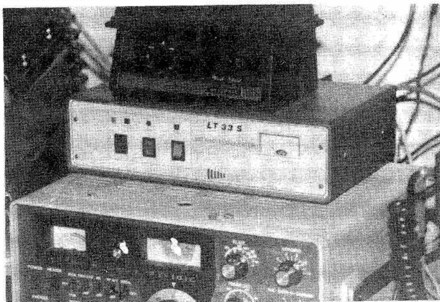
The LT-33 S transverter. This upconverts the 2-metre signals from the Icom IC-220A all-mode transceiver to 902 MHz.
