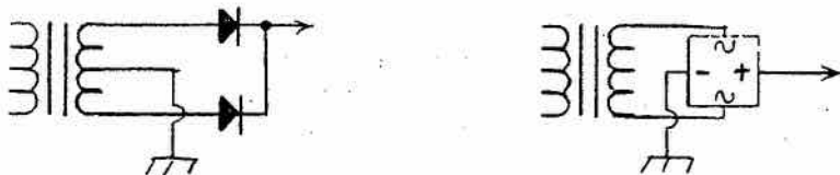
Fig. 3— Full wave diode and bridge circuits.
