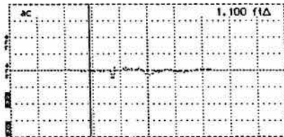
17. TV line cord, each line to ground compared differentially. Not such unbalance.
