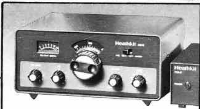
Microelectronics make the HW-9 QRP CW transceiver small and light.
