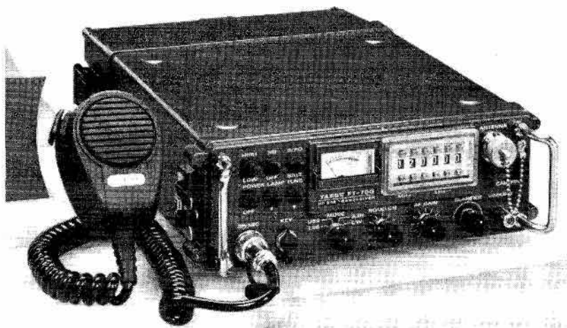
FT-70G Synthesized, full coverage, solid state, self-contained field portable
