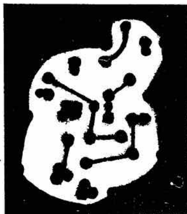
MODULATOR BOARD, FOIL SIDE.
