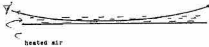
Figure 24: The heated air near the surface of a road bends the light waves from the sky up to your eye.
