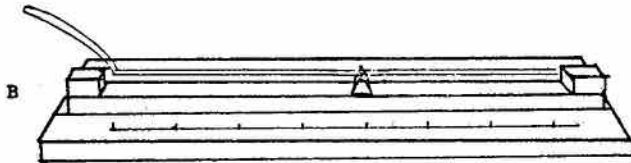
Figure 32b: The practical Lecher wavemeter.
