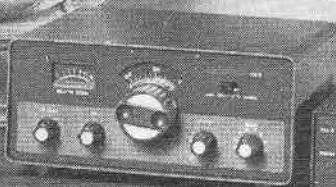
Microelectronics make the new HW-9 DSP CW transceiver small and light.
