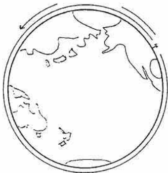
Figure 11: A radio signal completes a circuit round the earth (24,000 miles) in about one-seventh of a second.
