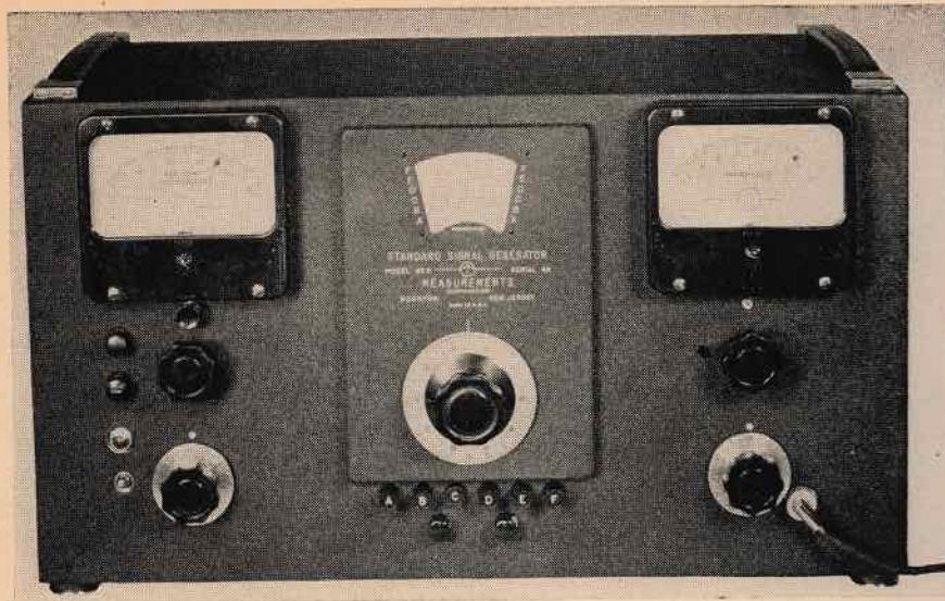
Fig. 2. Typical laboratory-type standard signal generator
