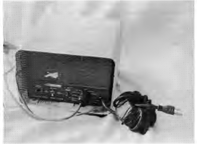
Figure 1—An effective way to decouple ac power cords for Field Day. The ferrite core is from the back of an old colour television picture tube. Another cheap source of ferrite cores: flyback transformers from a discarded television sets. But be careful retrieving it (see text)! The power supply shown is for a Heathkit SB-102 transceiver.
