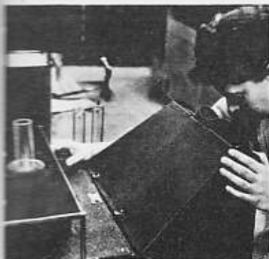
Seals between glass and metal parts are checked by polarized light, and by air under high pressure.
