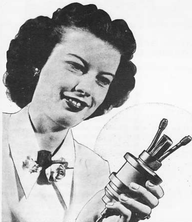
General Electric developed a new miniature magnetron for use, experimentally, in ultra-high-frequency television receivers, as well as in other equipment in which a low-power oscillator is required.
