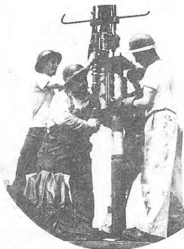
RCA engineers, working at a field laboratory near Camden, N.J., conduct tests on a model of the Empire State antenna.
