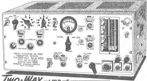
This is a single unit, crystal controlled, two channel set, with a frequency range of 3.0 to 6.3 megacycles. It was designed originally for use in fighter aircraft!! NOW - it's perfectly suited for 75 meter phone mobile operation, and a dozen other applications around the shack - for cottage and Field Day operation. A fine outfit.
