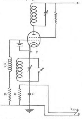
GM8RV's keying circuit; R1 is 10,000 ohms, and C1 .02 µF. It involves a small standing current on the valve to produce a self-biasing voltage.
