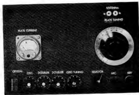
2. Front view of unit with all controls clearly marked. Meter is from captured German war equipment, but any small meter may be used in this application. Height of front panel may be reduced if desired.
