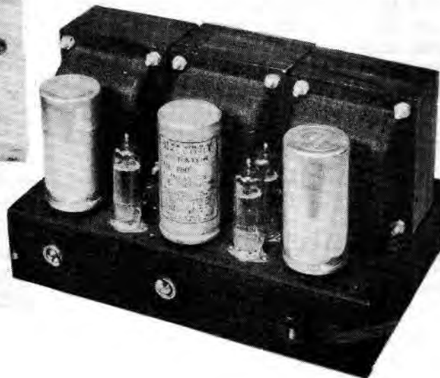
3. To the left - the top-of-chassis layout. At the extreme left of the unit are the plug in coils (see text), then the tuning gang, with the I.F.'s clearly shown. Wiring is straightforward. Note space behind panel available for batteries.
