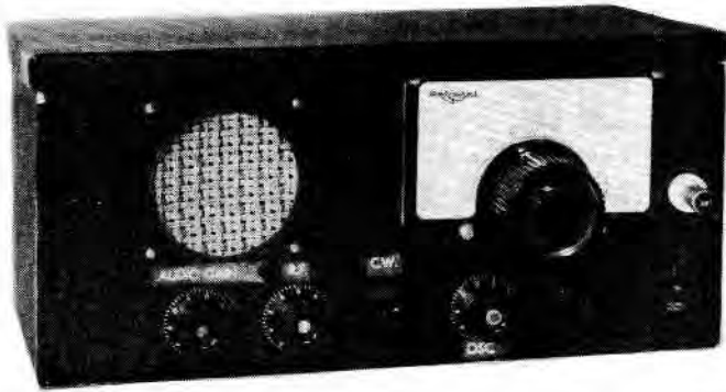
1. Front panel view of the completed receiver. To the left of and behind the speaker is the battery compartment (See 3) so that unit is completely self contained except for additional coils.
