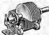
MC-1855—Double Bearing, Semi-Circular Plate. Capacity 100 mmfd. Air gap .024" \$2.21
