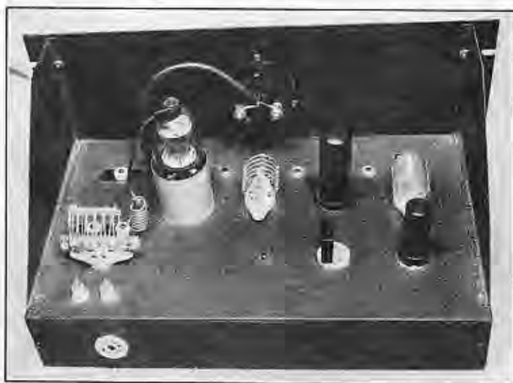
★ Top view of RF section. Isolantite insulation is used throughout. ★
